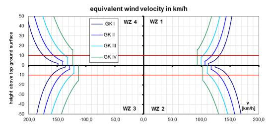
Figure 5: Conversion of the squall velocity pressures into equivalent wind velocities
