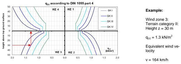
Figure 4: Graphic evaluation of the squall velocity pressures
